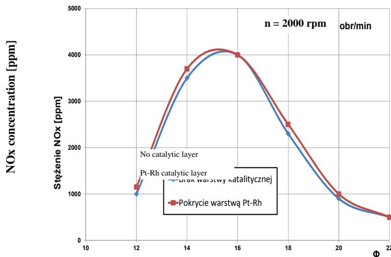
Fig. 4. NO<sub>x</sub> concentration change at engine speed of 2000 rpm due to the effect of the catalytic surface
