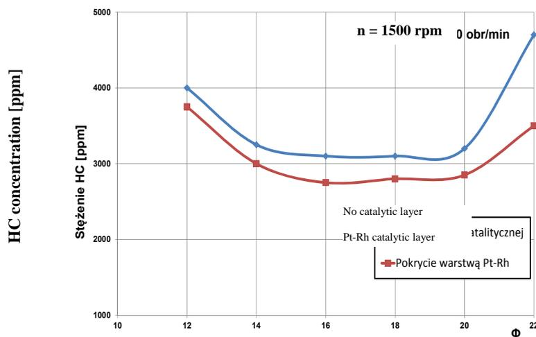
Fig. 1. HC concentration change at engine speed of 1500 rpm due to the effect of the catalytic surface
