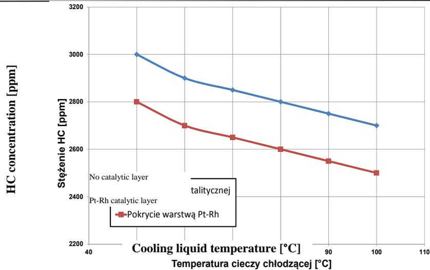
Fig. 5. HC emission change as a result of the catalytic surface at different coolant temperature values
