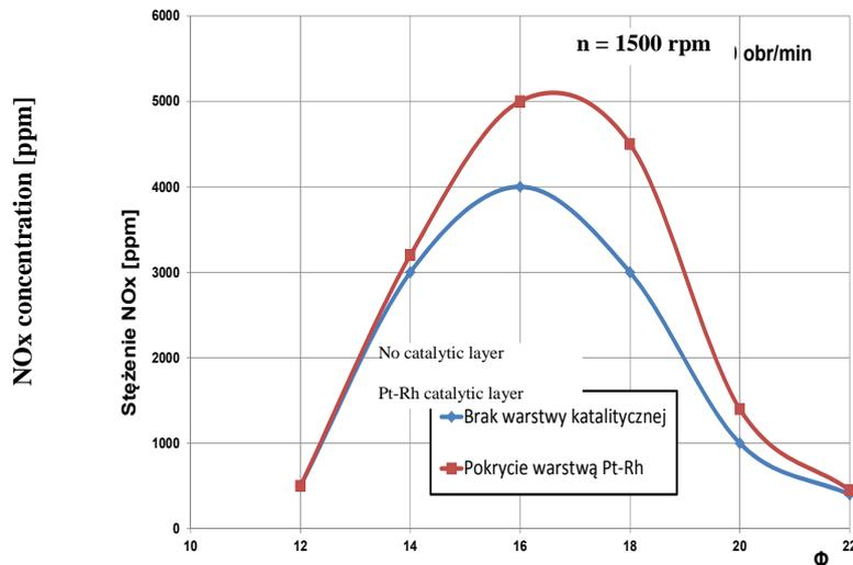
Fig. 3. NO<sub>x</sub> concentration change at engine speed of 1500 rpm due to the effect of the catalytic surface
