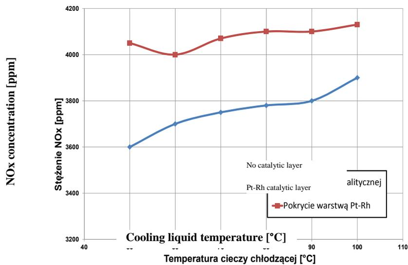
Fig. 6. NO<sub>x</sub> emission change as a result of the catalytic surface at different coolant temperature values
